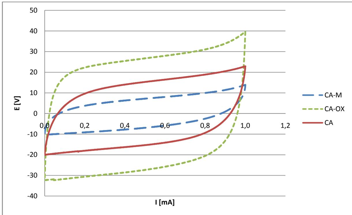
**Figure 1.** Cyclic voltammograms of carbon aerogels CA, CA-OX, and CA-M at 20 mV/s
