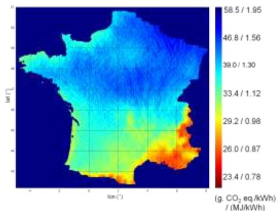
**Figure 2:** CO<sub>2</sub> production (g. CO<sub>2</sub> eq./kWh) and non-renewable primary energy use (MJ/kWh) for solar energy production depending on the level of irradiation over the French territory. (45° inclination + 25 years lifetime)
