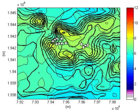
Figure 14: Horizontal wind speed resource at 60 m AGL for the Roussas wind farm computed from the centroid simulations. The colours give the wind speed in m s<sup>-1</sup>. Thick black lines are the orography contours. White stars give the wind turbine positions.
