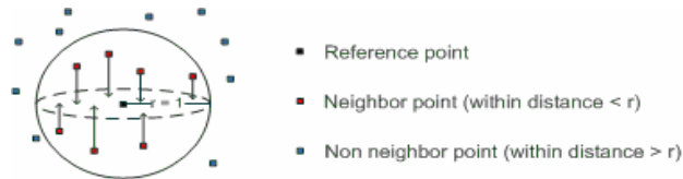
Figure 2 – Calculation of point density.
