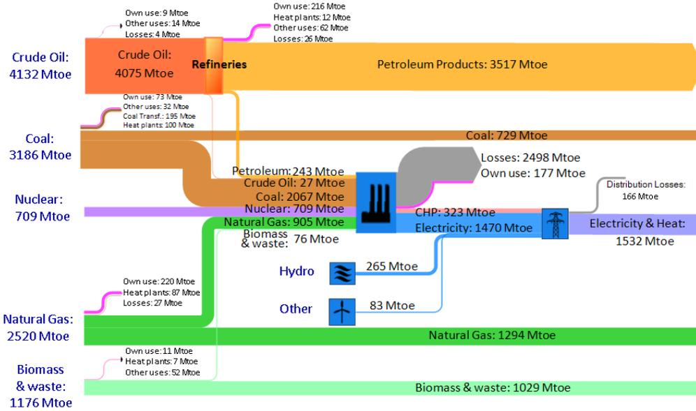
**Figure 2:** Energy supply-chain in Mtoe in 2007 (e!Sankey diagram). The electricity sector is severely disadvantaged by the efficiency of the Carnot cycle of the thermal units, and by the electrical losses at the transmission, distribution and consumption levels [5].
