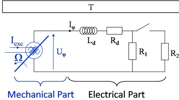
**Figure 5:** The one-loop grid, a circuit equivalent for a wide power system, described with a one-phase  $\varphi$  representation.  $U_\varphi$  is the voltage of the stator, i.e. the voltage supplied by the generator to the circuit.  $L_d$  and  $R_d$  are the inductive and resistive values of the transmission capacities.  $R_1$  models the load and connecting  $R_2$  models a load fluctuation.  $T$  is the thermostat considered in the thermodynamic framework.
