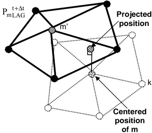
Figure 4. Projection of the centered position of  $m$  onto the patch  $P_{mLAG}^{t+\Delta t}$ .
