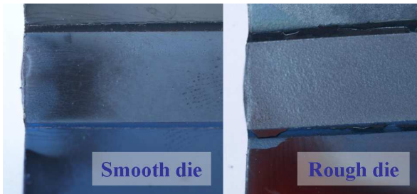
Figure 6: comparison of the oxide surface state after PSCT with rough / smooth dies. Die width 12 mm. \bar{\epsilon} = 0.4 , \dot{\bar{\epsilon}} = 1.s^{-1} , T = 900^{\circ}C , oxide thickness 50 \mu m .
