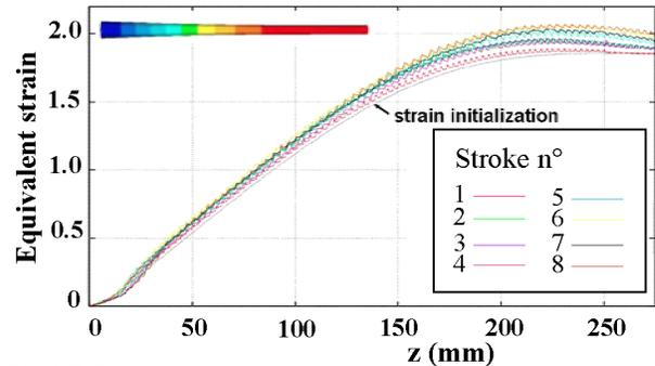
**FIGURE 4.** Progressive stabilization of strain along the “iterative” stroke computation process: the strain z-profile evolves from its initialization, shear-less guess to the final state. The insert represents the strain initialization, eq.(4) (blue:  $\bar{\varepsilon} = 0$  ; red:  $\bar{\varepsilon} = 1.8$ ).
