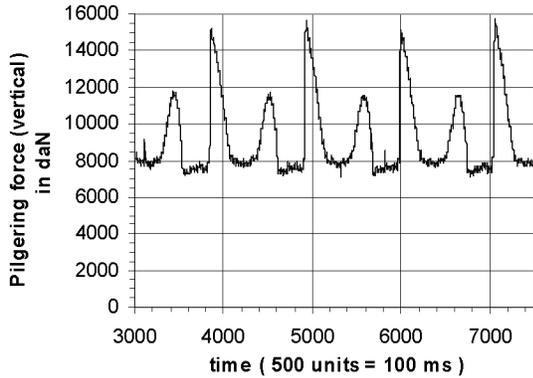
**FIGURE 3.** The measured pilgering force shows the periodic nature of the process. The minimum force (8000 daN) is a pre-compression imposed to the dies to avoid the “pilgering slit” (die separation changing the gap geometry).
