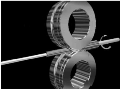
**FIGURE 1.** Principle of the cold pilgering process, showing the mandrel, the two dies (pictured here without their driving axes for better visibility), and the preform being pilgered (named “transition”).
