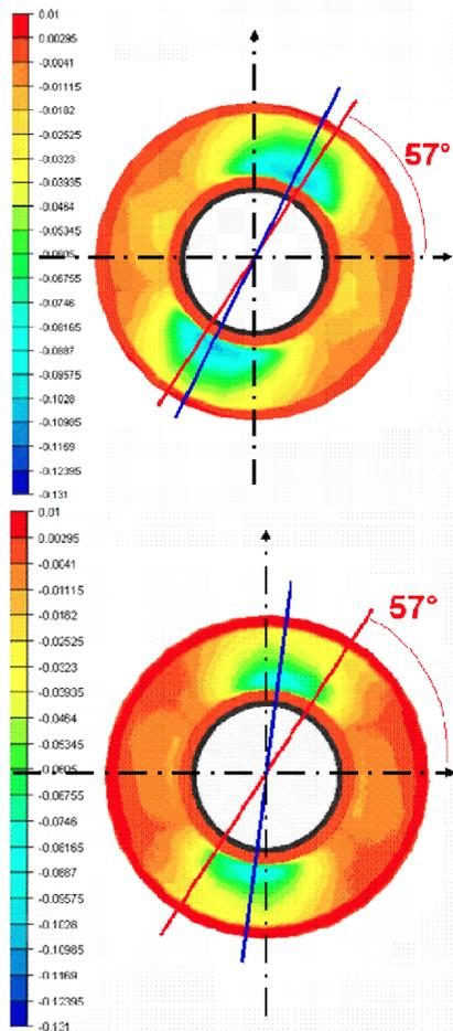
**FIGURE 5.** Progressive stabilization of strain along the “iterative” stroke computation process: the “transition” tube is seen from the front, showing the radial strain component on the external surface. Top: first stroke computation; bottom: 4<sup>th</sup> stroke. The thick blue lines points to the maximum radial strain.
