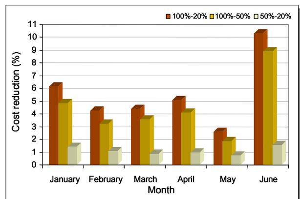
**Fig. 19:** Study on the power system of Crete. Estimation of monthly cost reduction due to improvement in the wind forecasts accuracy. A 6-10% reduction is achieved also in GHG emissions ( $SO_2$ ,  $NO_x$ ,  $CO_2$ ) by the use of an advanced forecasting tool that permits to avoid excessive reserves allocation.
