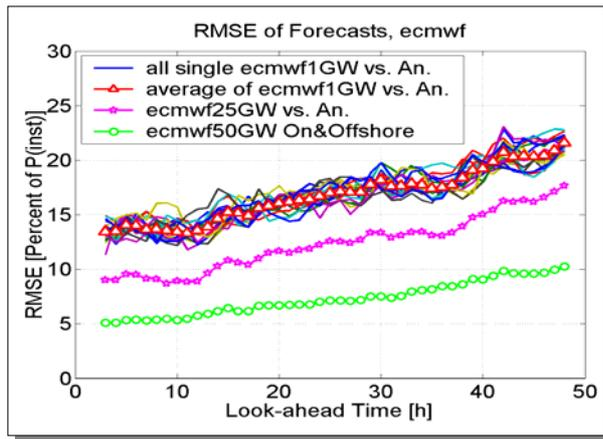
**Fig. 14:** RMSE of ECMWF wind power forecasts. Thin lines: all single 22 sites. Red triangles: Average of single sites. Pink stars: Aggregated 25GW offshore forecast. Green circles: Aggregated 50GW on-&offshore forecast.
