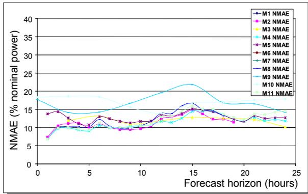
**Fig. 3:** Comparison of the performance of 11 prediction models on the Alaiz wind farm in Spain (very complex terrain). The NMAE is given as a function of the prediction horizon which here is 24 hours ahead.
