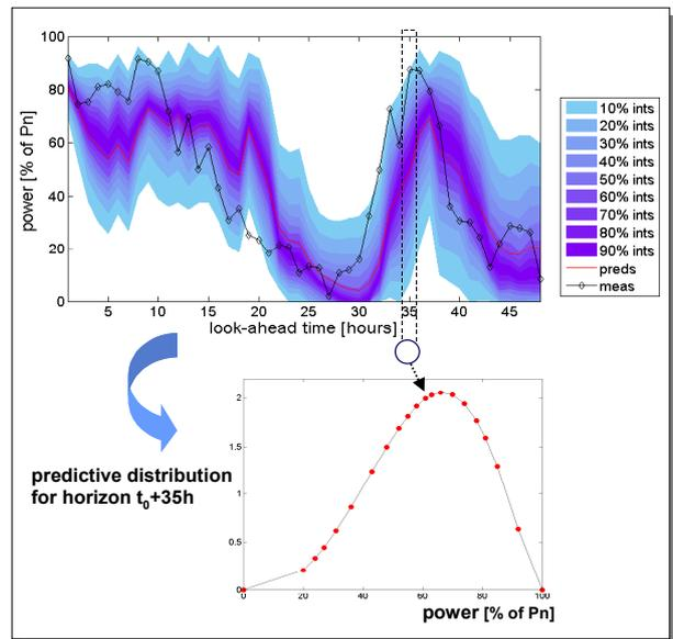
**Fig. 10:** Example of forecasts for the next 48 hours compared to measured values. Prediction intervals for various levels of confidence are displayed. Intervals are estimated with the adapted resampling approach.
