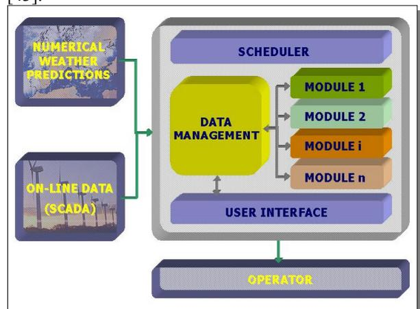
**Fig. 15:** General architecture of the ANEMOS prediction platform.
