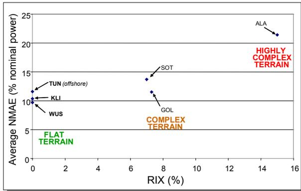
**Fig. 2:** Average NMAE for 12 hours forecast horizon vs RIX at each test case. Qualitative comparison. TUN is an offshore wind farm in Denmark, KLI is also located in Denmark, WUS in Germany, GOL in Ireland and ALA and SOT in Spain.
