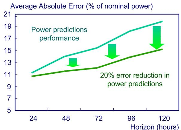
Figure 2: Improvement on average absolute error by using the Kalman filtering
