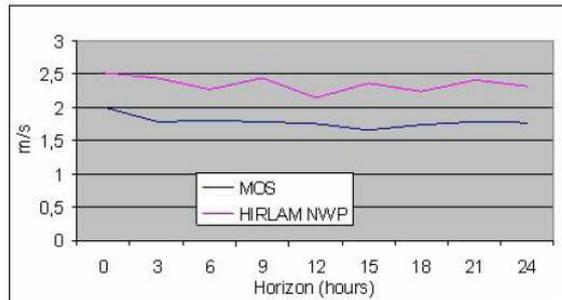
Figure 3: Statistical downscaling reduces forecast errors. The plot shows RMSE for forecasted wind speed at the Alaiz wind farm (ES) before downscaling (HIRLAM NWP) and after downscaling (MOS) for the 0.2° HIRLAM model.
