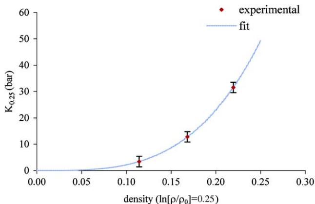
Fig. 2. Bulk modulus (at  $\ln(\rho/\rho_0) = 0.25$ ) as a function of aerogel apparent density.
