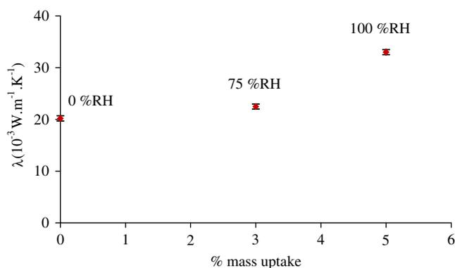
Fig. 7. Apparent thermal conductivity related to the sample mass uptake at different relative humidities.
