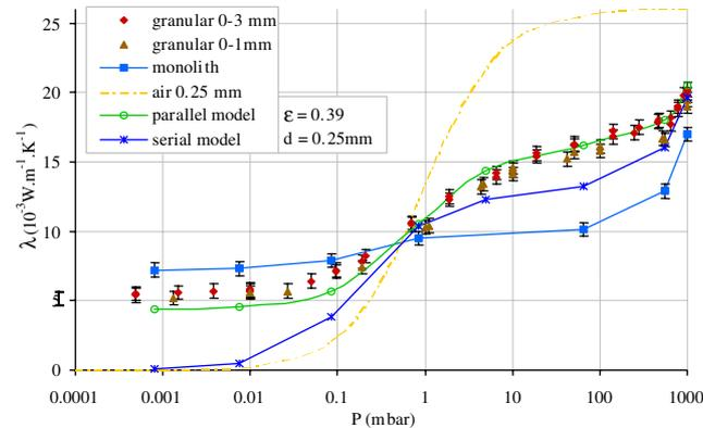
Fig. 6. Apparent thermal conductivity from  $4 \times 10^{-4}$  to 1000mbar for the different samples studied in this work, for air in 0.25mm voids (Eq. (3)) and for the calculated values to the serial and parallel models (Eqs. (4) and (5), respectively).
