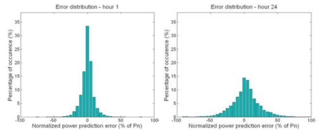
**Fig. 2.** The distribution of the prediction errors varies as a function of the prediction horizon (left picture: 1-hour ahead prediction error distribution, right picture: 24-hour ahead prediction error distribution). Results are produced using data for a single wind farm in Ireland.
