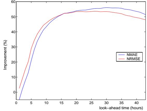
FIGURE 4: Improvement over Persistence obtained by an advanced model for both NMAE and NRMSE criteria.
