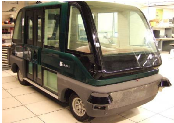
Fig. 5. Dual laser system of AGV.
