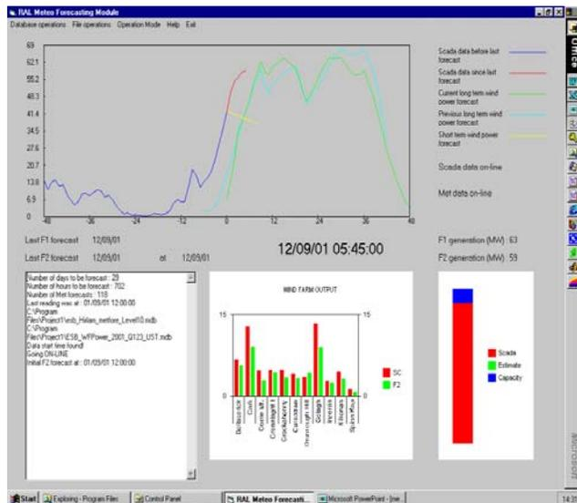
**Figure 5:** User Interface of RAL module
