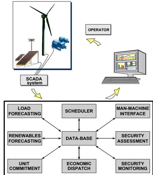
Fig. 1: The CARE system architecture.
