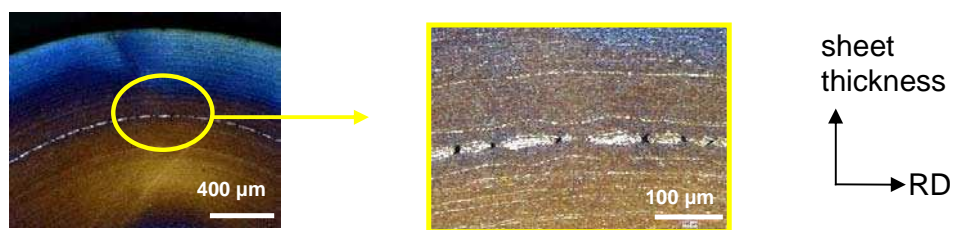
Fig. 6: Local necking around the central segregation band, optical micrographs, LePera etching
