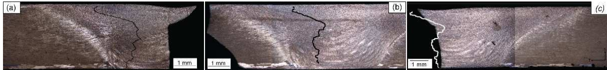
Fig. 10: Light optical micrographs of three representative welded fatigue specimens observed in the T-S plane for failure location (a) in weld nugget, (b) in TMAZ/HAZ, (c) next to the JLR. The JLR line has been redrawn for clarity in both three micrographs. Advancing side on the right
