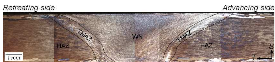
Fig. 4: Light optical micrograph of a JLR-free weld
