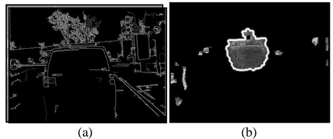
Figure 6. Illustration of the verification using lack of contours property. (a) is the sum of contours in frame  $n-1$  and  $n$ . Gray edges belong to frame  $n-1$  while white ones are from frame  $n$ . (b) As a result of the subtraction, only the connected component surrounded by white contours will be validated for further stages.
