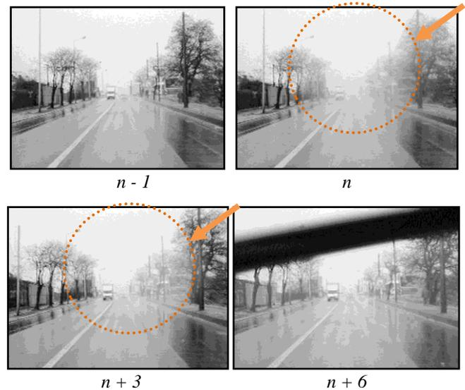
Figure 3. Evolution of an unfocused raindrop through the time starting at  $n$ . Frame  $n+6$  shows the wipers currently removing raindrops on windscreen. Raindrops are circled in light orange and image cropped for readability.
