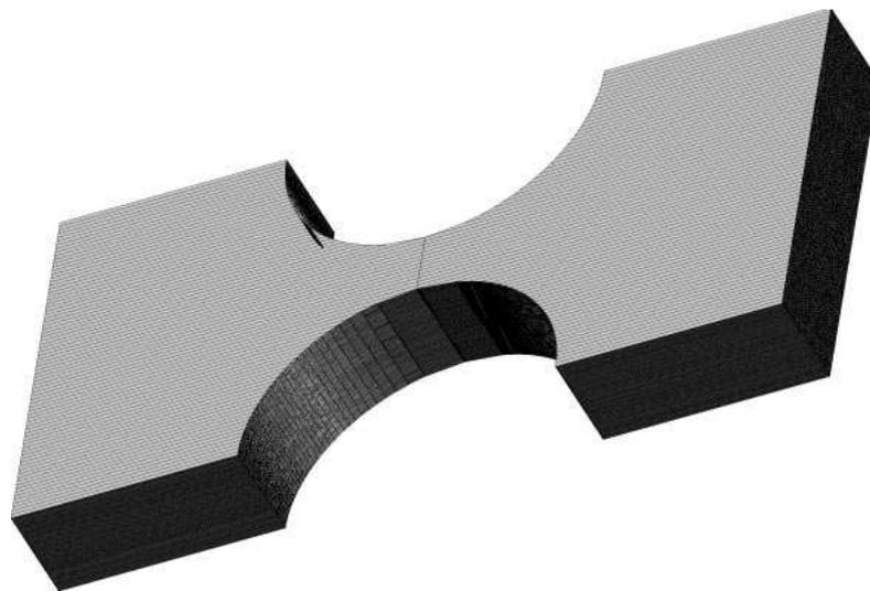
FIG. 9 – Mesh of the notched specimen.
