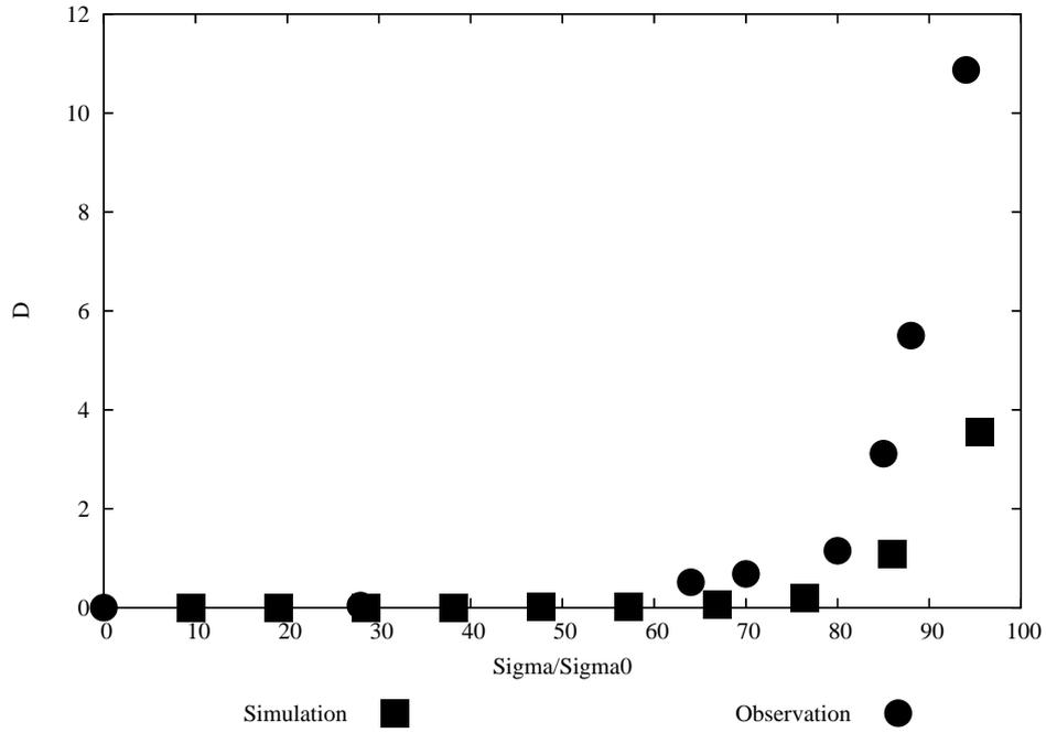
FIG. 7 – Density of fibre breaks ( $D$ ,  $nb/mm^3$ ) versus the increasing load ( $\text{Sigma}/\text{Sigma}_0$ ,  $\text{Sigma}_0 = \text{UTS}$ ). Comparison between observation and simulation.
