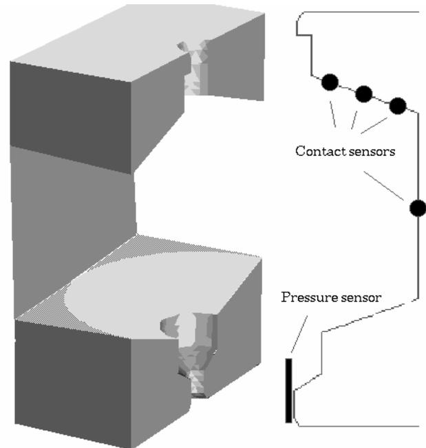
Figure 1. Instrumented mold.
