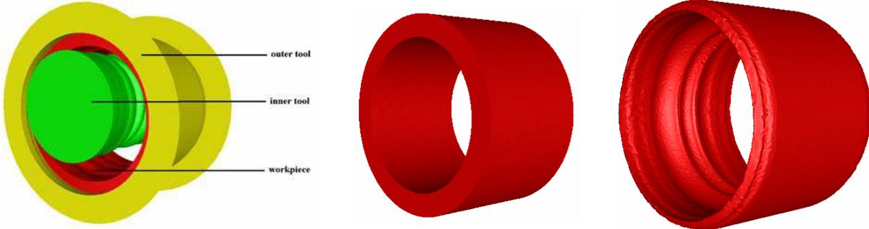
Fig. 7-1: ring rolling forging process      Fig. 7-2: ring at the beginning      Fig. 7-3: ring at the end
