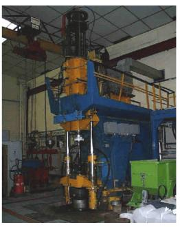
Figure 17: Full Scale Drilling Test stand
