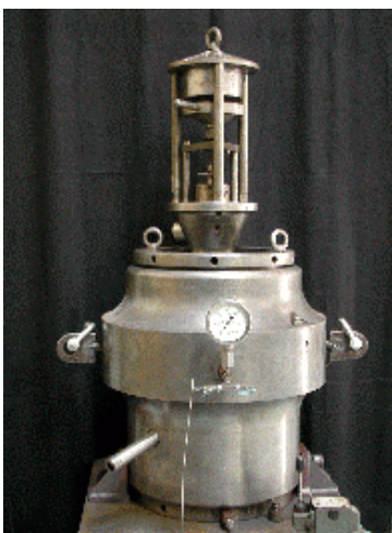
Figure 8 : confinement single cutter test stand
