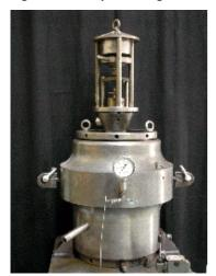
Figure 8 : confinement single cutter test stand
