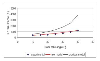
Figure 10 : PDC maximum normal force versus back rake angle
