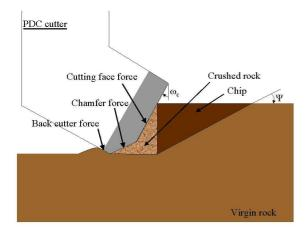
Figure 2 : Idealization of forces acting upon PDC cutter
