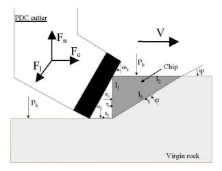
Figure 3 : build up edge of crushed material model
