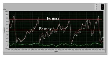
Figure 9 : Experimental PDC forces during rock cutting
