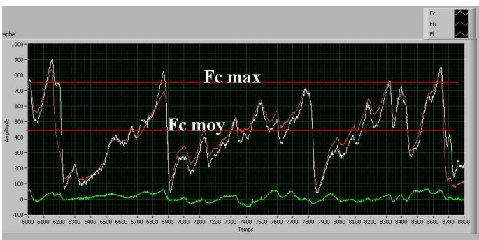
Figure 9 : Experimental PDC forces during rock cutting
