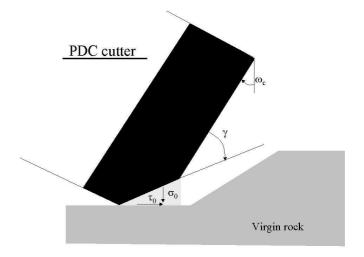
Figure 4 : Stress distribution within the chamfer zone
