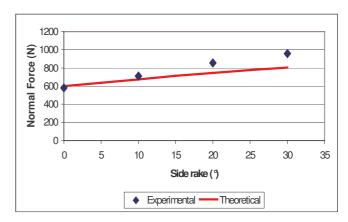
Figure 11 : PDC normal force versus side rack angle for asymetric cut
