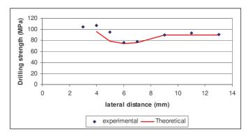
Figure 16 : drilling strength versus lateral distance to pre-existing cut for chamfered PDC
