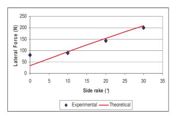
Figure 12 : PDC lateral force versus side rake angle for assymetric cut
