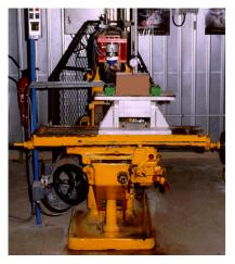
Figure 7: atmospheric single cutter test stand
