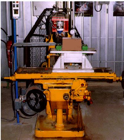
Figure 7 : atmospheric single cutter test stand
