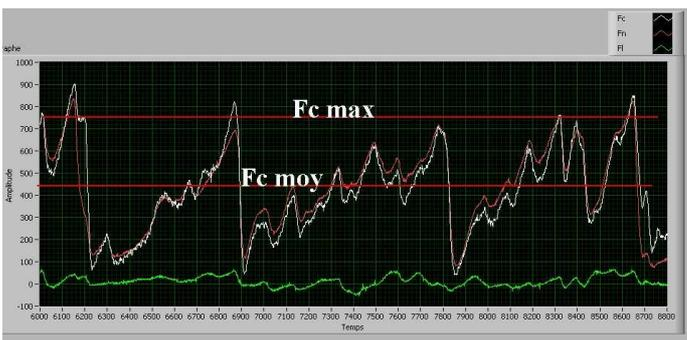
Figure 9 : Experimental PDC forces during rock cutting
