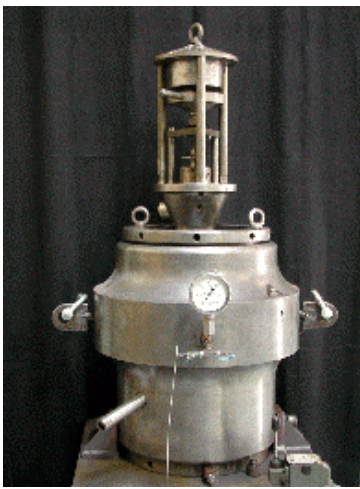
Figure 8 : confinement single cutter test stand
