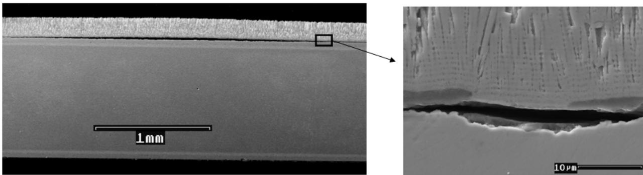
**Fig. 3:** Interfacial failure in TBCs due to LASAT
