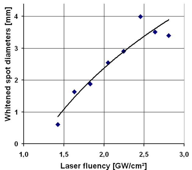
**Fig.4:** White spot diameter vs. Laser fluency plot for a LASATed TBCs (Ølaser=2.5mm)
