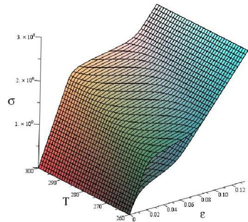
**Fig. 4** Surface of thermomechanical states,  $\sigma = f(T, \varepsilon)$
