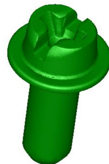
Figure 8: final Philips shape after forging
