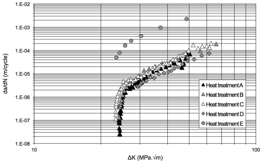
**Fig.4** Results of crack growth tests with dwell time at 650°C for the heat treatments investigated on SMO43.
