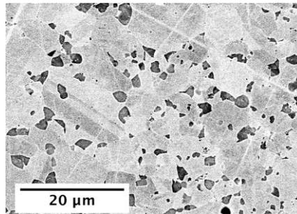
**Fig. 1** SEM micrograph (back-scattered electrons) of primary  $\gamma'$  precipitates from specimen subsolvus heat-treated.
