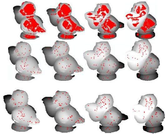
**Fig. 7.** Illustration of detectors stability, showing positions of detected keypoints (shown in *red*) for the views ( $100^\circ$ ,  $120^\circ$ ,  $140^\circ$  and  $180^\circ$ ) in bird model. Ligne 1: result of the connected components processes. Ligne 2, result of SC\_HK detector and ligne 3, result of SC\_HK\_FQ detector.
