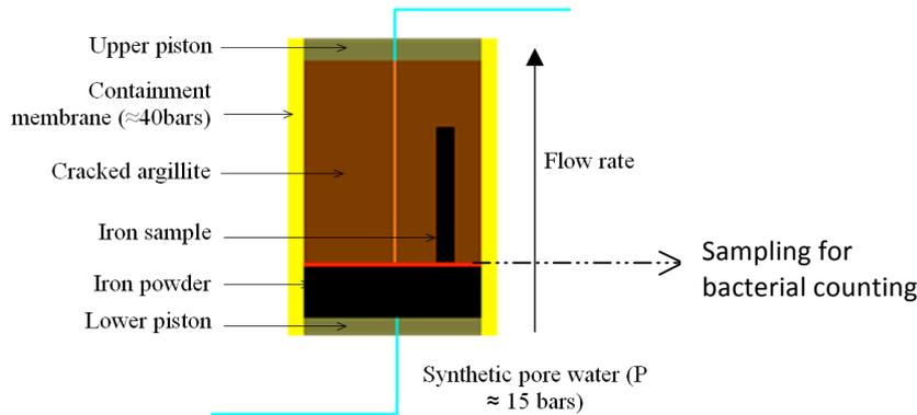
Fig. 1. Schematic view of the experimental cell
