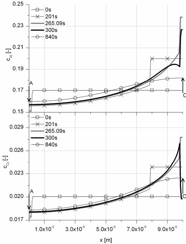
Figure 2: Concentration profiles during the solidification and dissolution/homogenization heat treatments.
