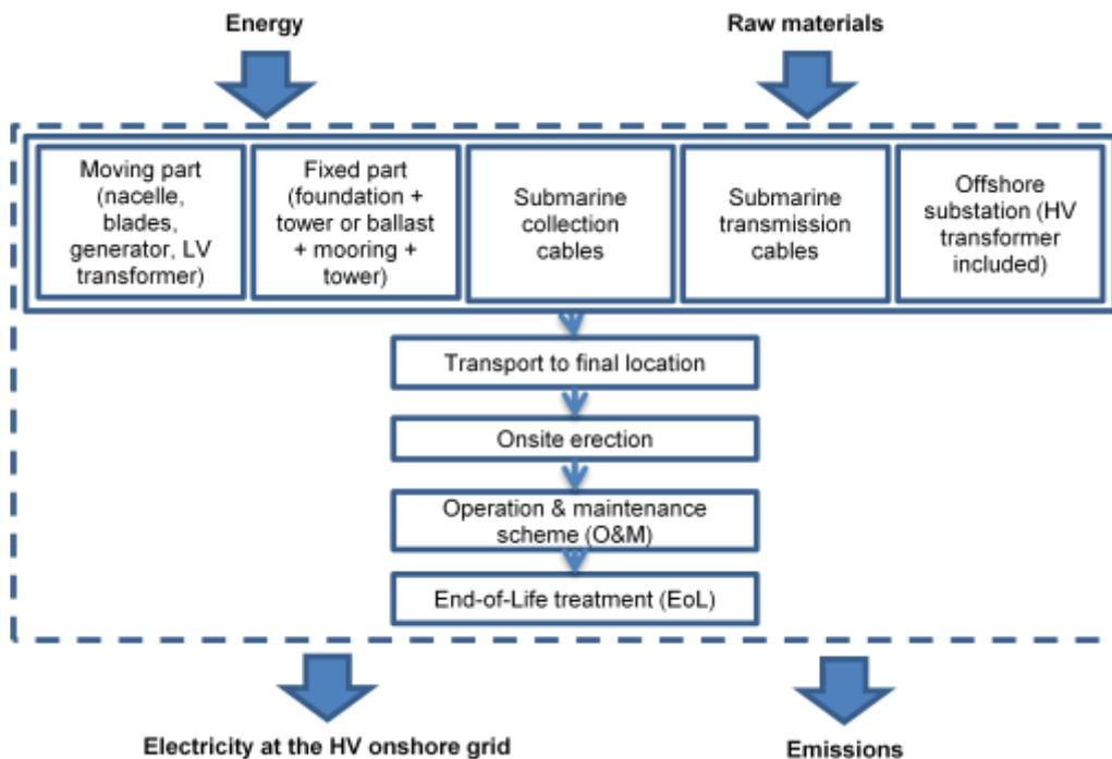
Figure 1: Components considered for the offshore modular LCA model
