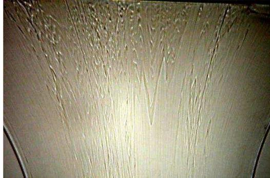
Figure 1: Characteristic defect on an industrial coextrusion line
