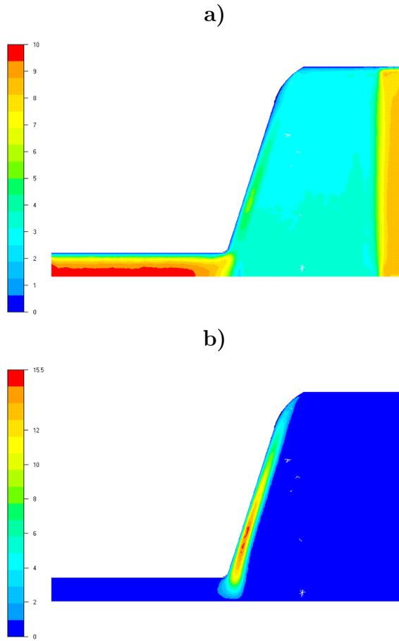
Figure 5: Mid-plane velocity field ( $cm/s$ ) in the flow direction (a) and in the transverse direction (b) (the flow rate is  $1.10 cm^3/s$  and density  $\rho = 1.33 kg/dm^3$ ).
