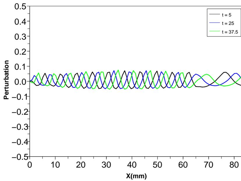
Figure 11: Spatial evolution for various time steps of relative perturbation for a forcing frequency of  $1\text{ Hz}$  in the outlet zone; processing conditions correspond to the unstable experimental case 4
