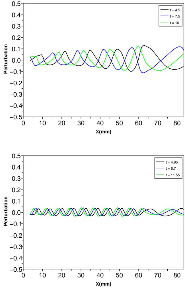
Figure 15: Case N<sup>o</sup> 4 and 30° angle in the convergent geometry. Perturbation along flow motion for various time steps; a) forcing frequency 0.5 Hz, b) forcing frequency 1 Hz
