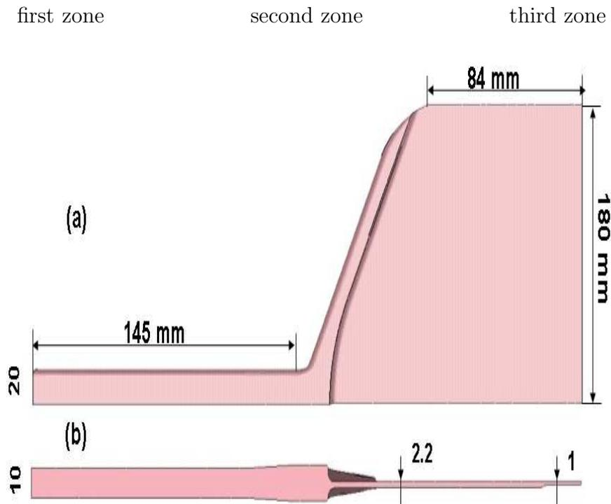
Figure 2: View from the top and through the thickness of the coat-hanger geometry: (a) 1/2 die and the three different areas ; (b) view in the thickness direction along the symmetry plane
