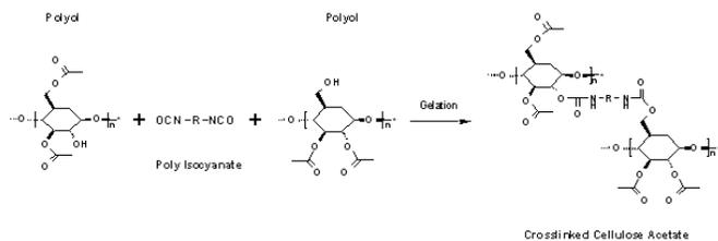
**Figure 1.** Scheme of urethane crosslinking of cellulose acetate.
