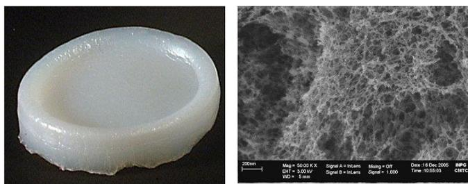
**Figure 2.** Aerogel (left) and its SEM-FEG micrograph (right).
