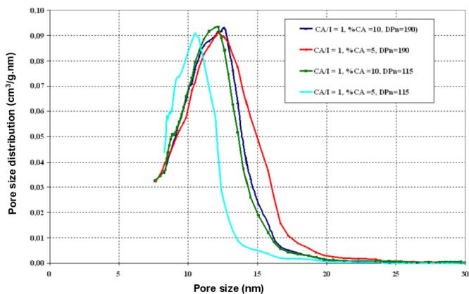
**Figure 3.** Pore-size distributions of aerogels prepared with CA/I = 1 characterized by non-intrusive Hg porosimetry<sup>14</sup> with  $k_f = 28$  nm.MPa<sup>1/4</sup> ( $d_{Hg}$  and % $V_{Hg}$  were also characterized with this technique).
