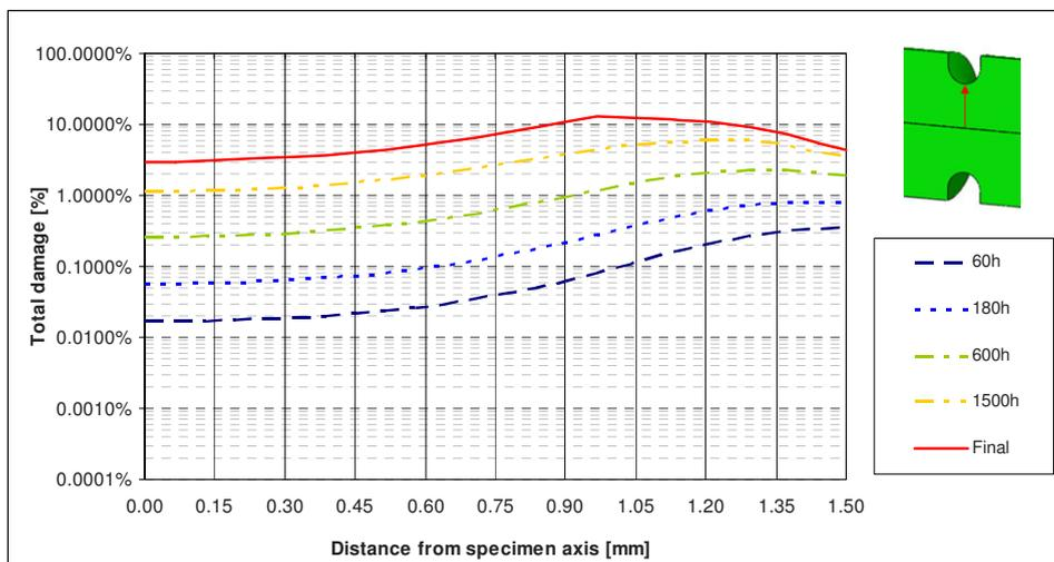
Fig. 6. Progressive development of the creep damage towards the centre of the sample during the test notched sample NTCD0.6M under 240 MPa at 600°C.
