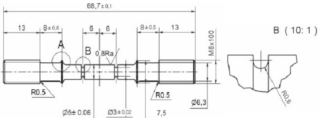
Fig. 4. Dimensions (mm) of notched creep samples (NTCD0.6M).
