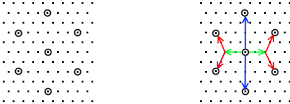
Figure 12: Initial structuring element used to compute sparse conjugate hexagons (left). This structuring element is obtained by combining shifts (in green) and supFarNeighbor operators (in red) on the hexagonal grid with supFarNeighbor transforms (in blue) on the square grid. Note that the size of this structuring element is 2).
