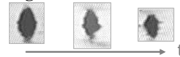
Illustration of the erosion mechanism for the N234 carbon grade ( R_0 = 22 \mu m ) in SBR under shear ( 6 s^{-1} ).
