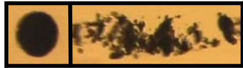
Figure 3: illustration of the fragmentation mechanism for a silica agglomerate with an initial radius of 37 \mu\text{m} at 56s -1
