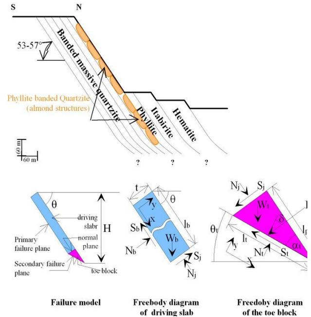
Figure 9 : South slope face of the Timbopeba mine in Brazil: bilinear slab potential failure mechanism
