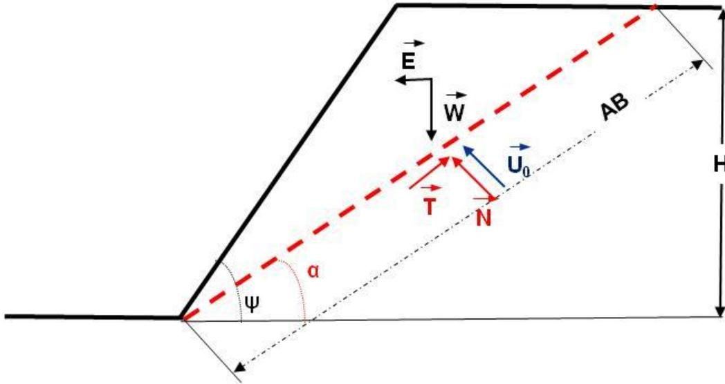
Figure 1: Equilibrium of a block sliding on a plane failure surface
