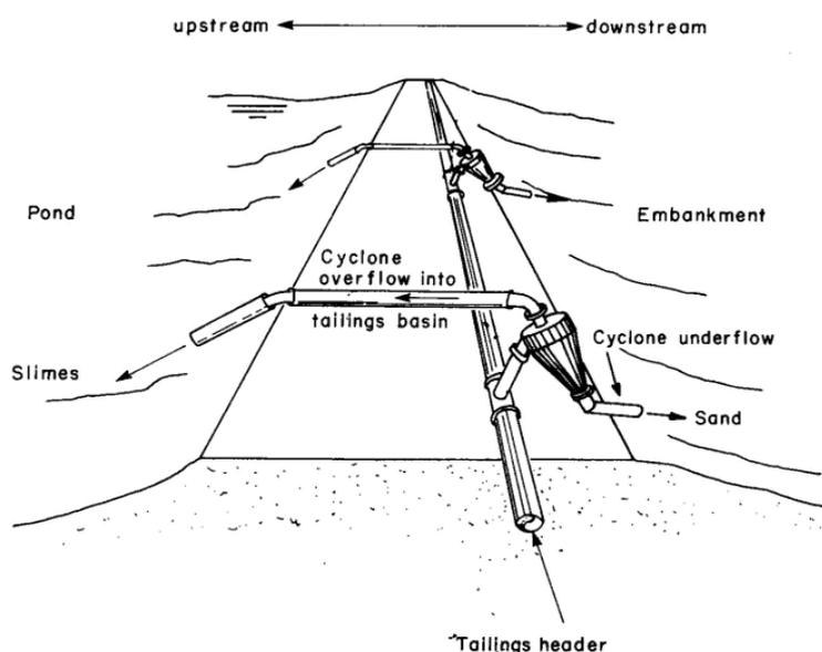
Figure 11: Typical hydrocycloning arrangement (after ICOLD, 1996)
