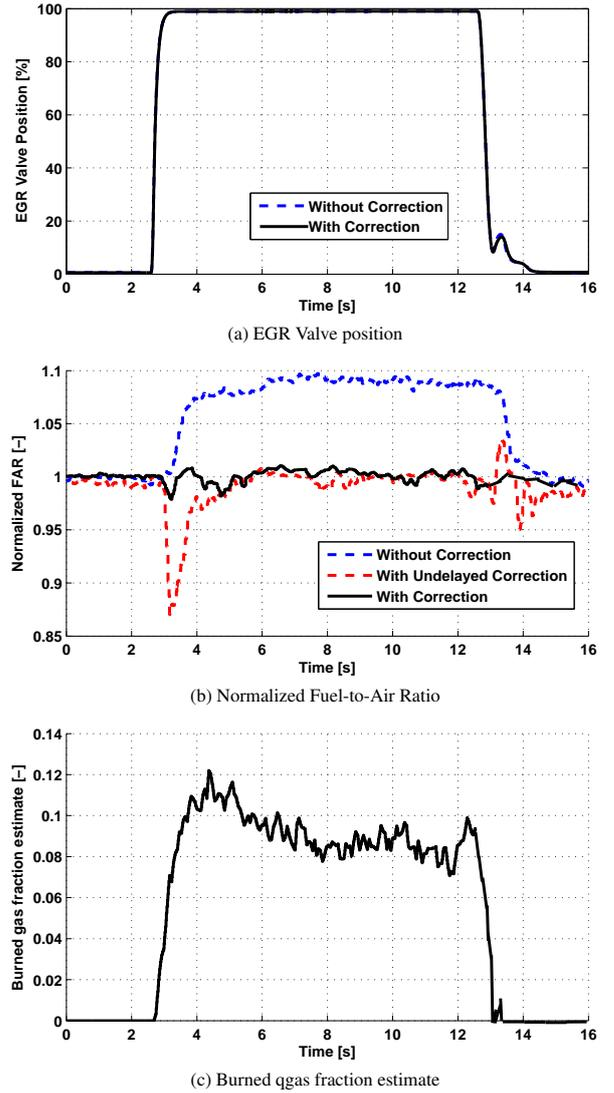
Fig. 6. Experimental results for constant engine speed ( $N_e = 2000$  rpm) and torque request ( $IMEP = 8$  bar). The EGR valve position is pictured in (a). Blue dotted curve : gas composition transient without estimation. Black curve : gas composition transient with estimation and feedforward correction.
