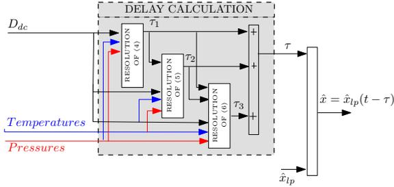
Fig. 4. Scheme of the proposed delay calculation strategy for intake burned gas fraction estimate  $x$ . The numerical solving of implicit integral equations (4)-(6) can be obtained by sampling and calculating the integrals at increasing values of  $\tau_i$  starting from 0, which are real-time compliant calculations.
