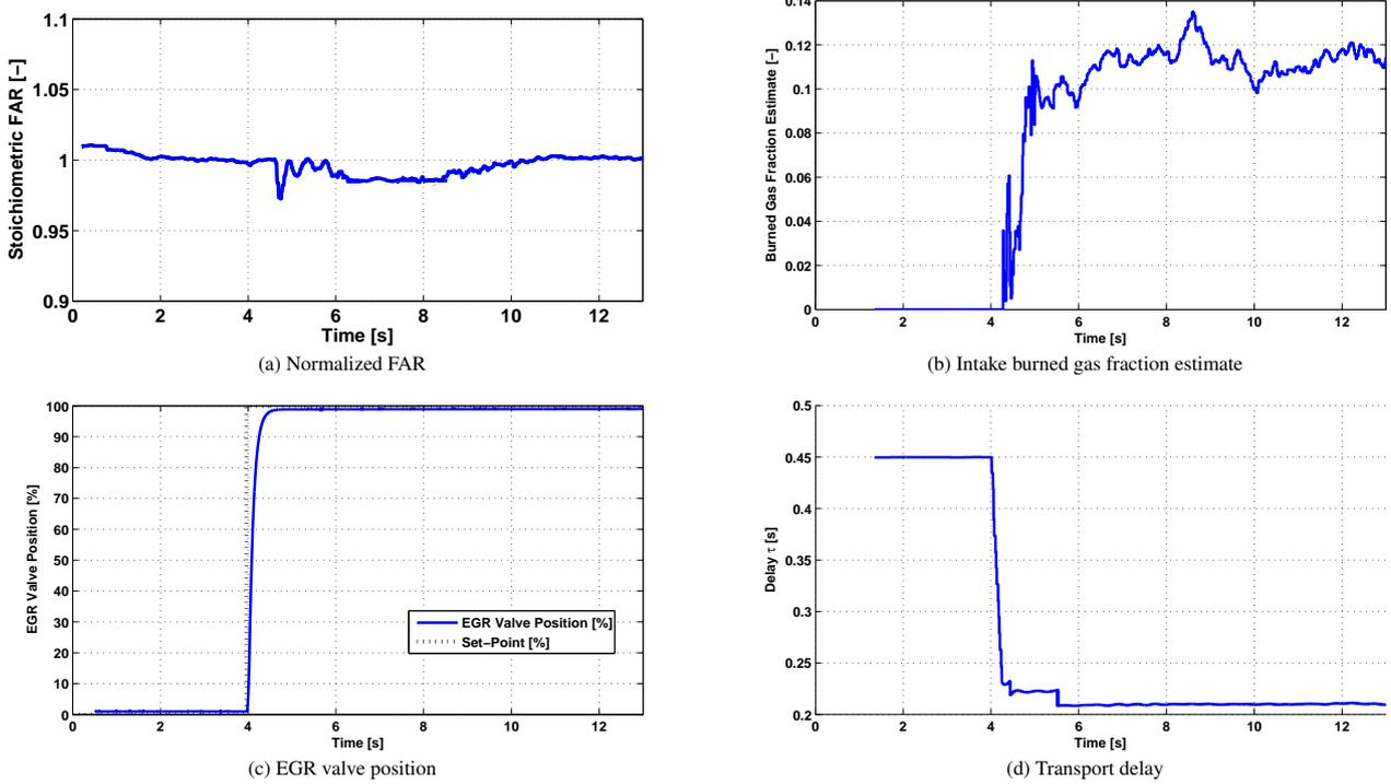
Fig. 7. Experimental results for constant engine speed ( $N_e = 2000$  rpm) and transient torque request (step from  $IMEP = 6$  bar to 12.5 bar), resulting into a delay variation. The normalized FAR response pictured in (a) uses the intake burned gas fraction estimation pictured in (b), obtained with the on-line estimation of the delay (d).
