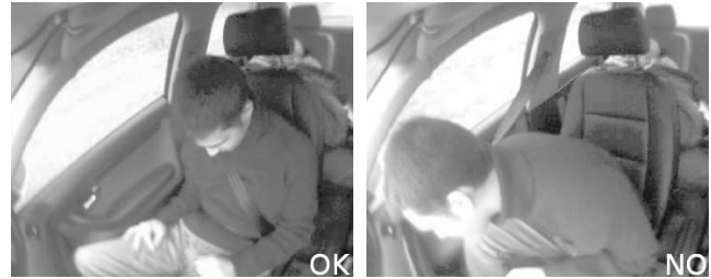
Figure 2. Out of position ( OOP ): airbag ok or not
