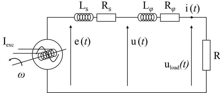
Figure 2: Single-phase representation of the one-loop circuit.
