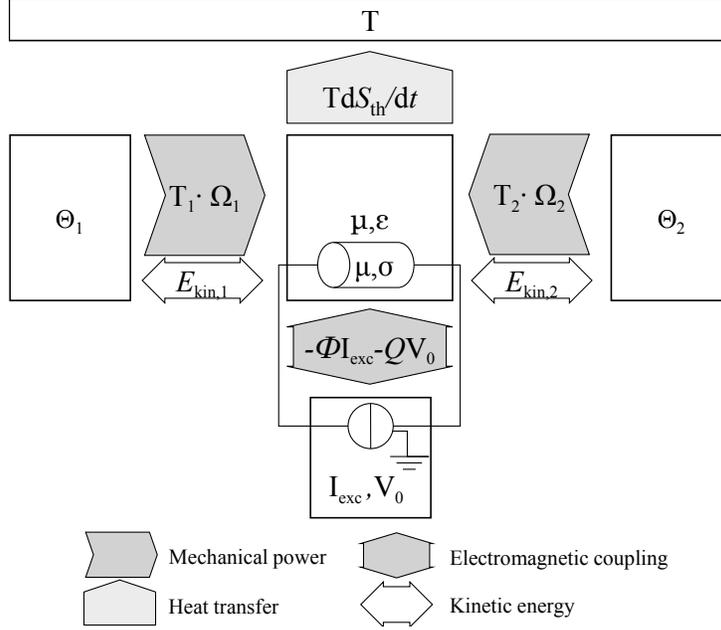
Figure 1: Chart of the energy exchanges between the subsystems involved in the thermodynamic representation of a power system [33, 34].  $(\mu, \epsilon)$  and  $(\mu, \sigma)$  respectively described conductors and dielectrics immersed in the electromagnetic field conveying power between the subsystems. Arrows illustrate the power exchanges.
