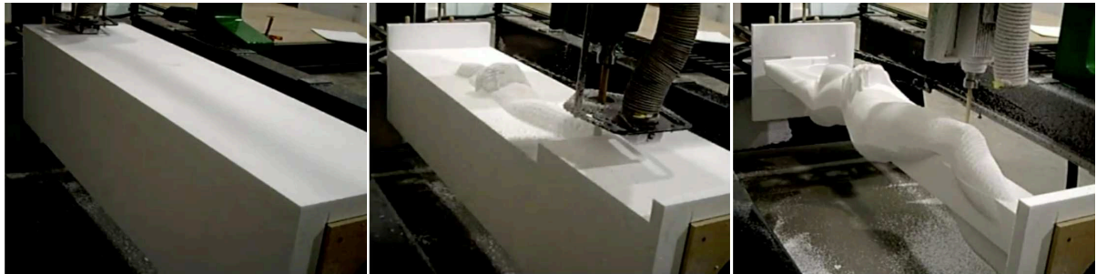
Figure 3. The transformation of some input material by a CNC machine via a set of planned actions.
