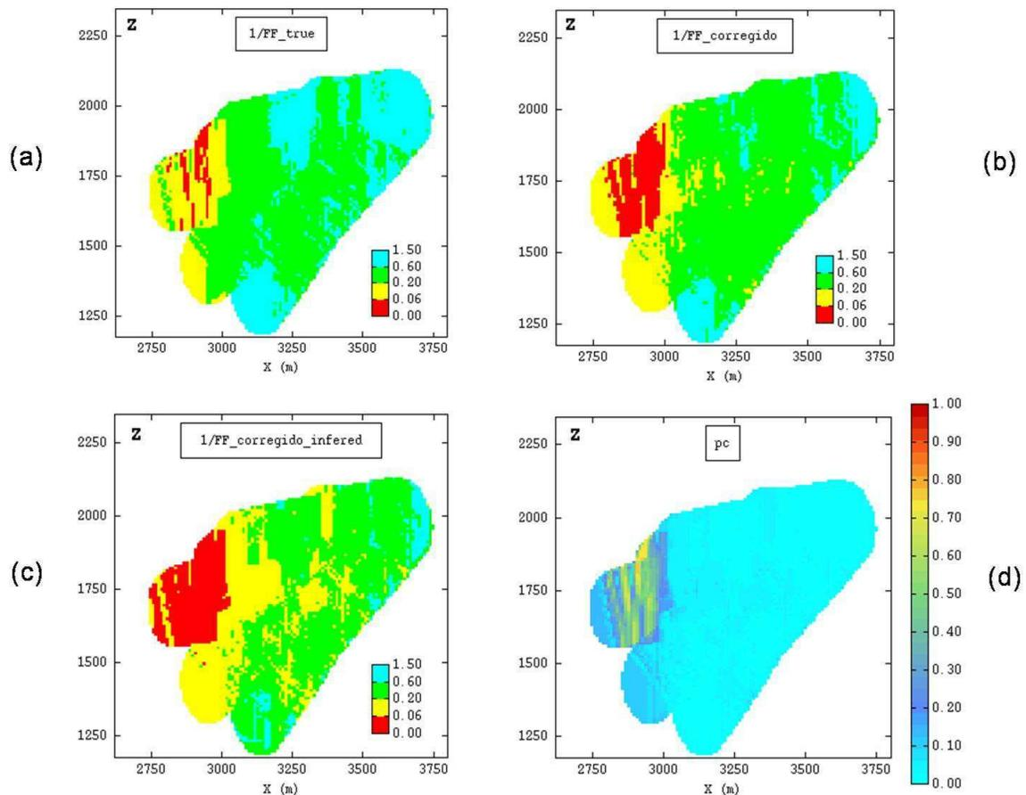
**Fig. 5** (a) Map of inverse True Fracture Frequency using block kriging. (b) Map of inverse Usual Fracture Frequency that incorporates crushing estimate and arbitrary frequency for crushing equal to 40. (c) Same as (b) but with crushing frequency inferred from statistics and set to 80. (d) Crushing proportions at block scale estimated by kriging
