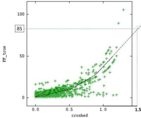
**Fig. 6** Scatter diagram between crush length ( $L_C$ , horizontal axis) and  $FF_{\text{true}}$  as defined by (1). Solid line represents the conditional expectation curve; dotted segment represents a conservative extrapolation
