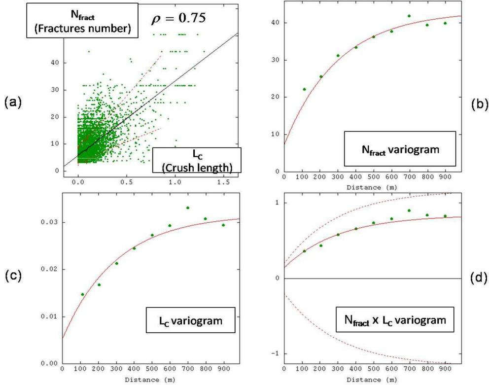
**Fig. 4** (a) Scatter diagram between crush length ( $L_c$ , horizontal axis) and Fractures number ( $N_{fract}$ ). Line represents the linear regression of  $N_{fract}$  against  $L_c$ , as well as the conditional expectation curve. Red dotted lines represent the standard deviation around the conditional curve. (b-c-d) Resp.  $N_{fract}$ ,  $L_c$ , and  $N_{fract}$  cross  $L_c$  variograms. Points are experimental, continuous curves the intrinsic model (all the variograms are proportional)
