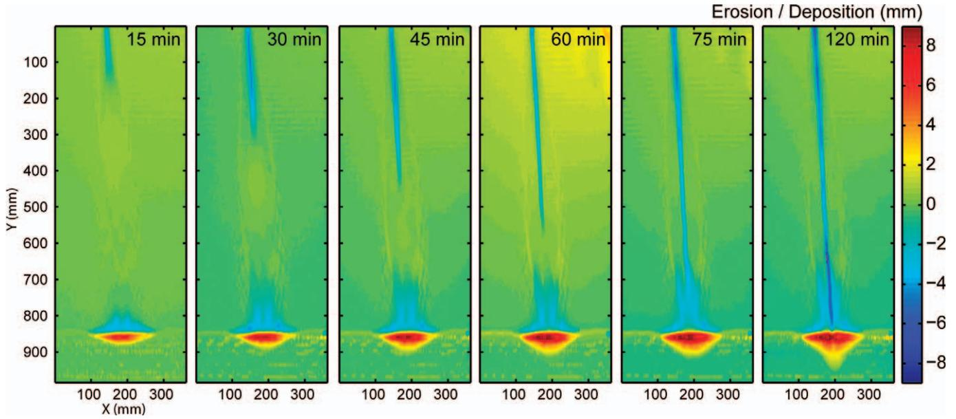
FIG. 6.—Map of the cumulated erosion and deposition for experiment Exp\_10 (initial slope  $10^\circ$ , input discharge rate  $40 \text{ mL}\cdot\text{min}^{-1}$ ). 75 minutes after the beginning of the experimental run, the topography has almost reached steady state and sediment transport has virtually vanished. Erosion is represented in cold colors, and deposition in warm colors.
