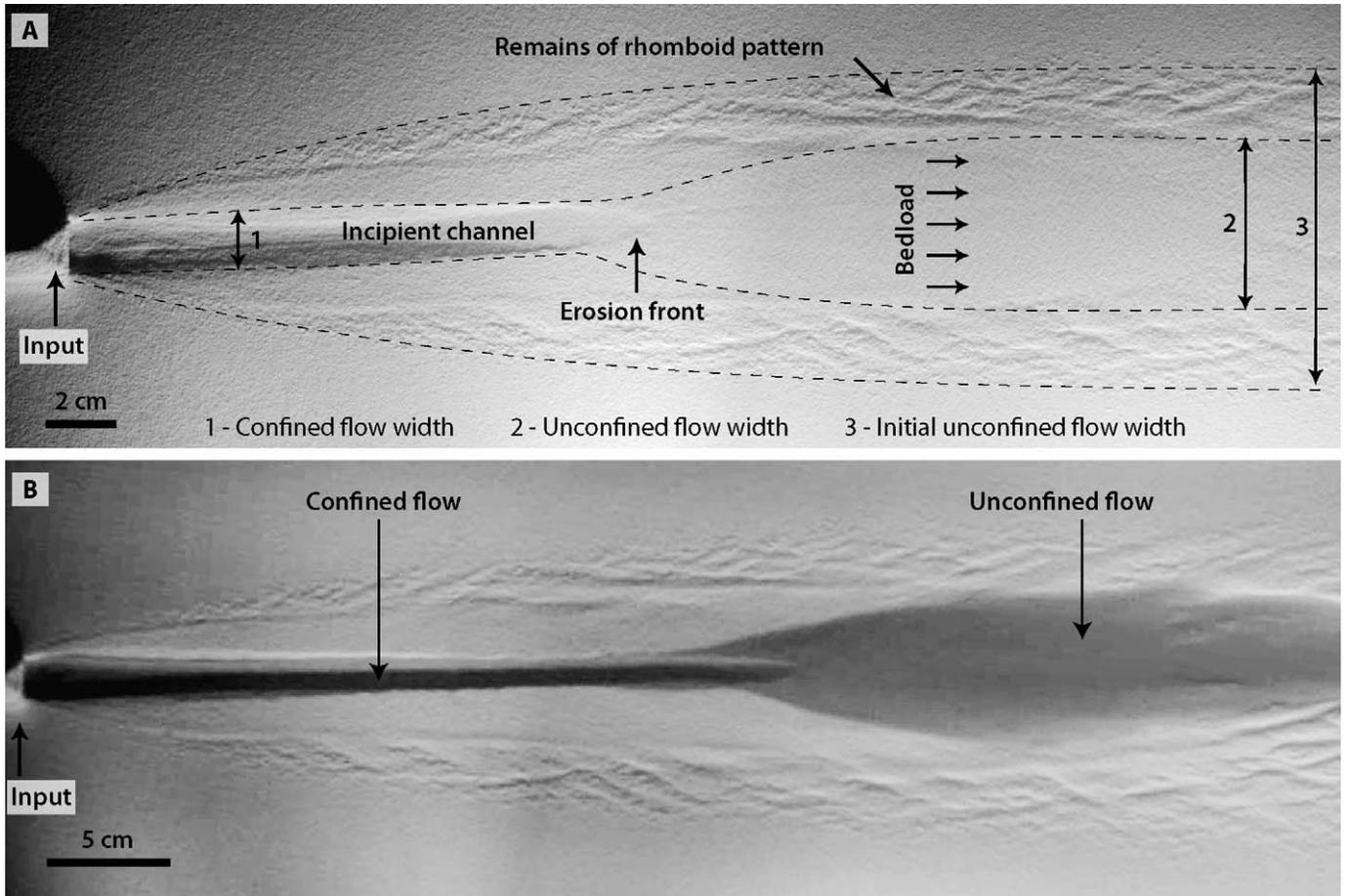
FIG. 4.—Downslope propagation of the channel (flow is from left to right): **A**) 20 min after the beginning of the experiment and **B**) 40 minutes after the beginning of the experiment. In the second picture, the gravity current is visualized by injecting dye in the brine. Exp\_04: discharge = 40 mL·min<sup>-1</sup> and slope = 8°.
