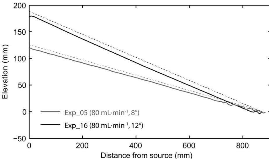
FIG. 9.—Longitudinal profiles of channels at steady state for two runs (Exp\_05 and Exp\_16) with identical discharges but distinct initial slopes. Dashed lines represent initial bed surfaces before the beginning of the channel incision.
