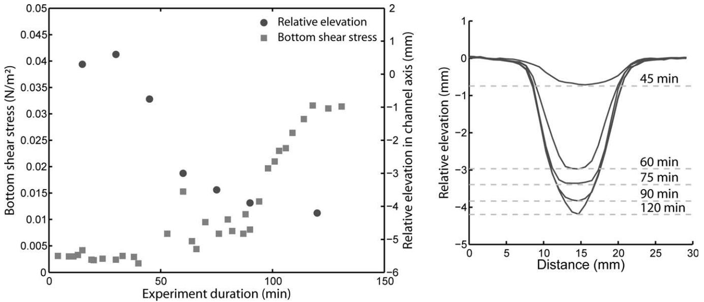
FIG. 8.—Evolution of bottom shear stress and channel depth through time for Exp\_10 ( $40 \text{ mL}\cdot\text{min}^{-1}$ ,  $10^\circ$ ). Left: Bottom shear stress and channel depth measured at 50 cm from the inlet. Right: Evolution of the channel cross section at the measurement location.
