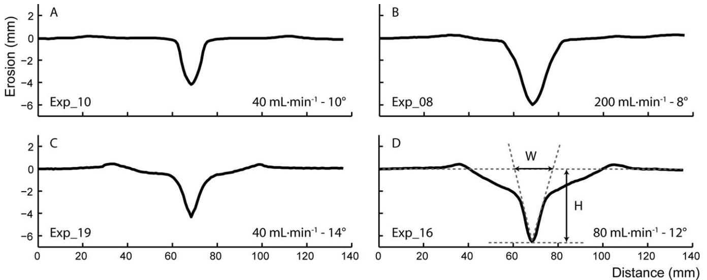
FIG. 10.—Steady-state cross-section average over 220 profiles for four different experiments: **A, B**) Single-phase channel incision at low slope values, **C, D**) Two-phase channel incision at high slope values. The definitions of both the channel width and depth are illustrated in Part D.
