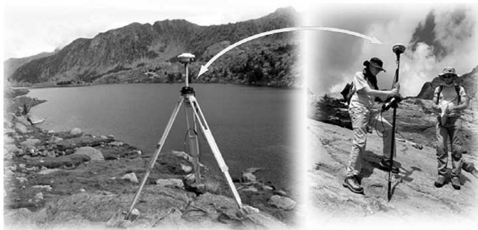
Fig. 1 – Base station receiver at the Lac Long Supérieur, mobile receiver in the valley.
