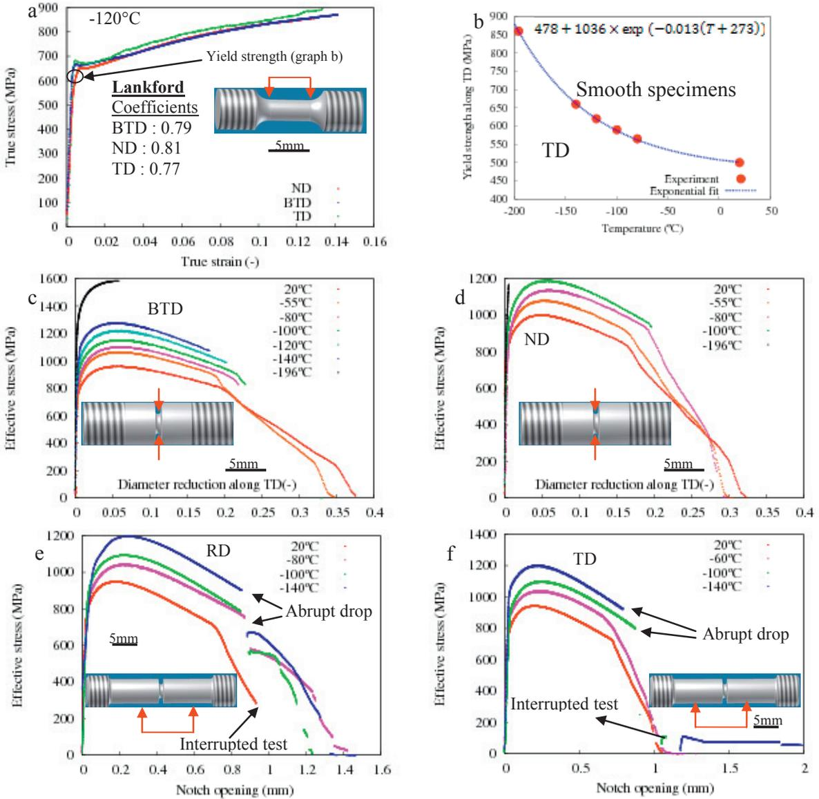
Fig. 2. (a) Tensile curves from smooth specimens at -120°C; (b) Evolution of yield strength with temperature; (c-f) Tensile curves of notched specimens. Red arrows indicate the location of extensometers ends.
